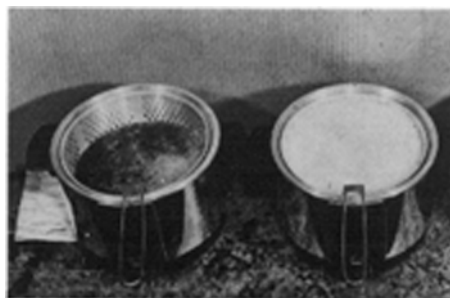
FIG. 2. When potato slices were deep-fat fried in fresh corn oil (left) and in corn oil which had been heated at 185 C for 72 hr (right).
